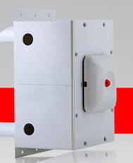
The duct smoke detector YKB02 is designed to detect the presence of smoke in airstream of ductwork sections or ventilating compartments by the smoke detector mounted in it.
