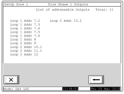
If no addressableoutputs are associated to the zone, a screen with the message *No addressable outputs activated upon Fire Condition Phase X* (X stands for phase number – 1 or 2)
