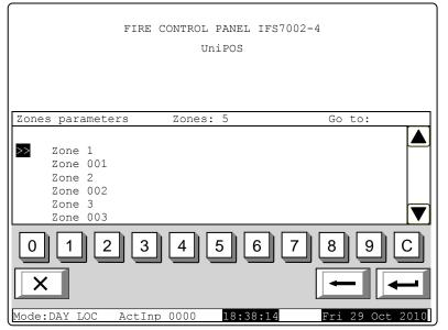
Buttons and allow the used to select the next or the previous zone (if any are available). When you press a digit button, the field *Go to* is activated and a random 3-digit number designating the zone number can be entered in the field. To edit the 3-digit number, press button and you can delete the last entered digit.
