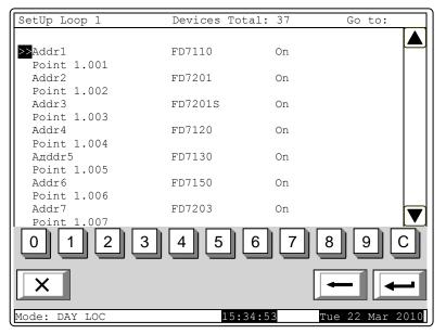
and the digit buttons appear if more than 7 devices are available in the loop. Press a digit button, the *Go to* field is activated and a random 3-digit address for each device in the loop can be entered.
