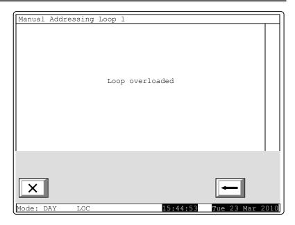
In case of short circuit in one of the loop lines or in case of straight loop (the message in the bottom right corner appears in case of short circuit in one of the loop lines only):
