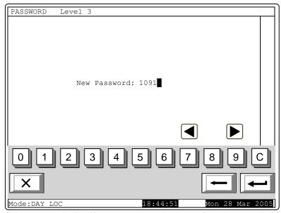
The maximum length of the password is 10 symbols. If you press a button after the 10-digit password is entered, the exceeding symbol will not be accepted.
