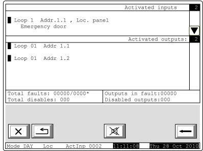
Use the buttons | and | in the right part of the panel to display the next screen with activated outputs if their total number for the output is greater than 4.
