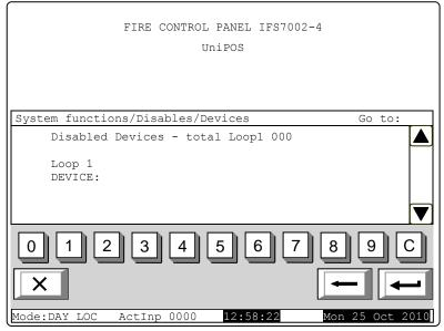
If disabled addressable detectors are available – the first disabled fire detector, and in the bottom section of the panel appears the detector's text message:
