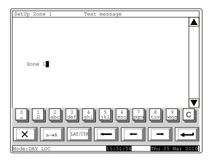
during this 1 second, the cursor first moves one position to the right and then the new symbol is inserted. The maximum length of the message is 40 symbols. If you press a button after a 40-symbol message is already entered, the text will not be accepted and the symbol will not be inserted (the cursor moves one position to the right if the end of the text message is not reached yet).
