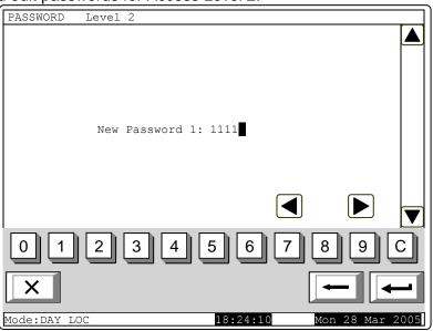
The maximum length of the password is 10 symbols. If you press a button after the 10-digit password is entered, the exceeding symbol will not be accepted.
