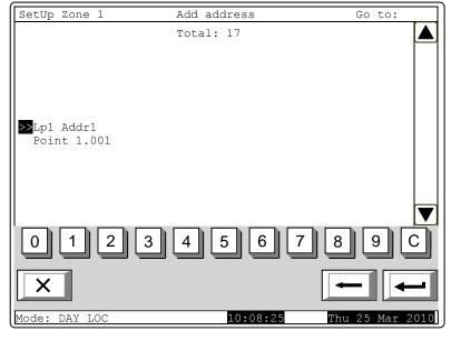
When you press a digit button, the *Go to* field is activated; you can enter a random 3-digit number for a device in the field. To edit the number push button C, and the last inserted digit is deleted.
