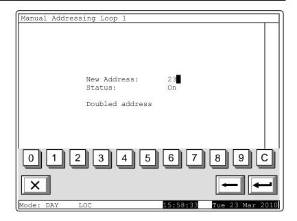
\* Where no device with the same address is detected and the operation is successful, it will proceed to the next uninitialized device, if any, or the screen from section 5.2. will be displayed.
