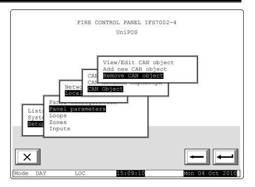
The Screen shows the total number of the connected objects and their list. In the list, each object is identified by name and CAN address.
