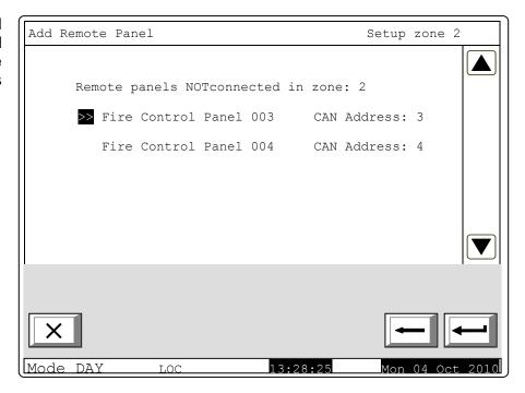
After selecting the Remote Panels, served by that zone go to menu "Maintenance Remote Panels" where appears a window Select Remote Control Panel, by means of which zones will be served.
