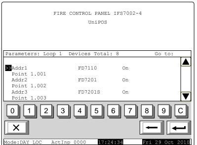
If the device is FD7201 or FD7201S type and we want it to operate as a monitored input, enter Settings /Loop / Loop X / Device Parameters and proceed as follows for FD7201 type to be setup as a monitored input:
