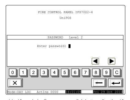
The maximum length of the password is 10 symbols. If you press a digit button after the 10-symbol password is entered, the digit is not accepted and will not be entered.
