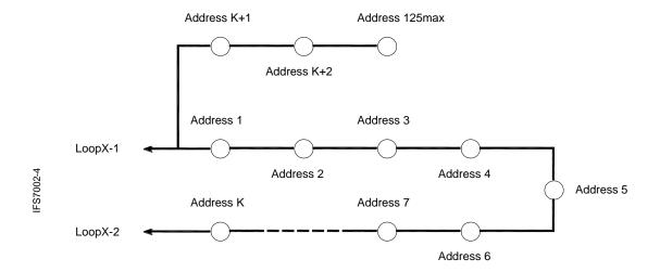
d) Improper connection of Fire alarm loop branch (the branch is connected between the control panel and an addressable device)
