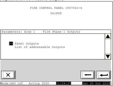
The screen *Panel Outputs* provides information for outputs responding to the relevant phase of Fire condition in the zone:
