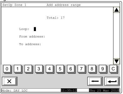
Press button to add the free devices in the group to the zone; the limit of 60 devices in a zone is accordingly observed. The following information is displayed:
