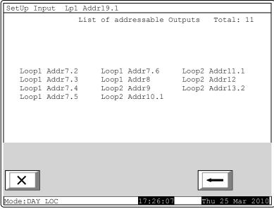
If no addressable outputs subject to activation through the addressable input are available, a screen with the text message *No addressable outputs activated by this Input* appears.
