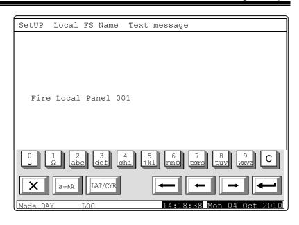
After reverting to the main menu you may continue the configuration of the local parameters. The screen displays the name of the local Control Panel (in the initial start up of the Control Panel, that name is factory set.)
