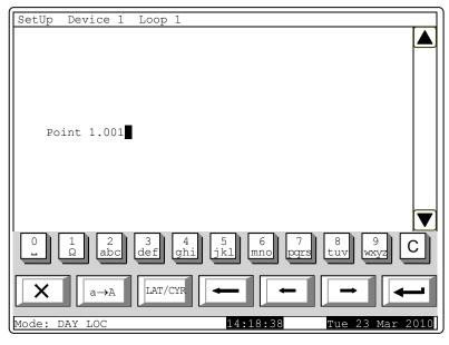
If you press another button during this 1 second, the cursor first moves one position to the right and then the new symbol is inserted. The maximum length of the message is 40 symbols. If you press a button after a 40-symbol message is already entered, the text will not be accepted and the symbol will not be inserted (the cursor moves one position to the right if the end of the text message is not reached yet).
