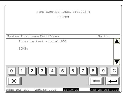
If some zones in test are available, the first zone in test will be displayed, and in the panel bottom section will appear the text message of the zone:
