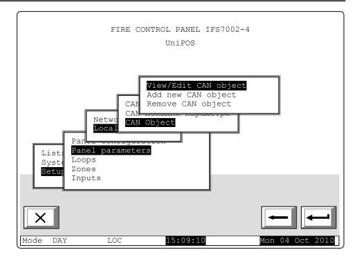
Choosing the option above allows for reviewing and adjustments through the menus similar to those described above. Example: The screen shown contains information three connected for objects. By scrolling choose which object to be reconfigured.
