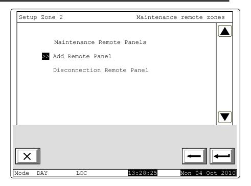
First add (select from the Remote Panels already entered) to the Remote Panel. Upon entering the Menu, a list of all Remote Panels, connected to this Control Panel and their addresses on the network is displayed.
