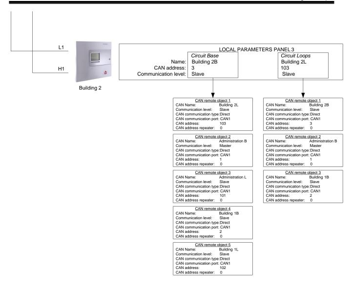
**5.2.** Example of a network of Remote Control Panel for Indication and Control IFS7002R and three 4-loop Control Panels of IFS7002.
