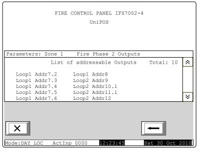
The buttons  $\stackrel{\triangleright}{}$  and  $\stackrel{\triangleright}{}$  on the right panel section appear where more than one page is available and allow the user to switch between next and previous page.
