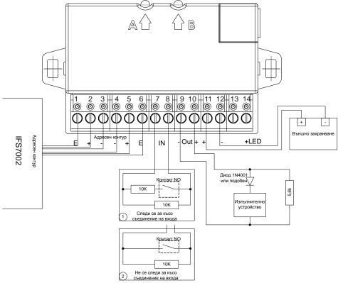
Input-output device FD7203 (1 input/1 output-monitoring)
