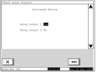
Upon exit of the menu the activated relay output is switched off.
