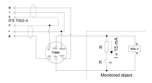
FD7201 connected to monitored input
