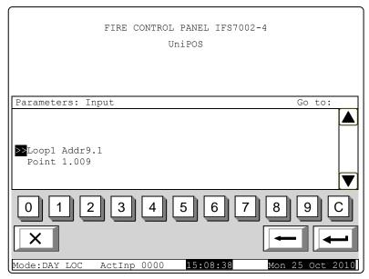
Buttons and seen on the right panel section appear when more than one addressable input is available; the Go to field and the digit buttons appear when more than one addressable input device is available.
