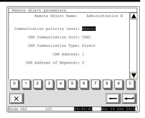
the relevant control panel shall be defined. Also, the connection type shall be changed, in **CAN Communication port**: **Via repeater**. Repeater's address shall be set too – as a CAN address of an object –repeater. The repeater object shall be described as an object assigned to the CAN, to the local control panel.
