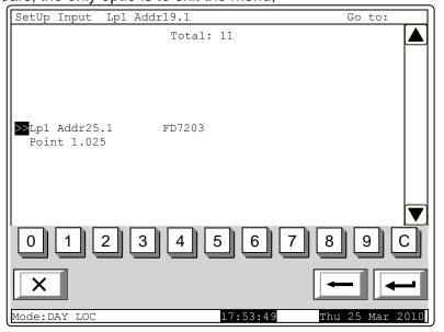
Buttons and in the right panel section are visualized if more than one free addressable output is available, the Go to field and the digit buttons appear if free addressable outputs in more than one module are available.
