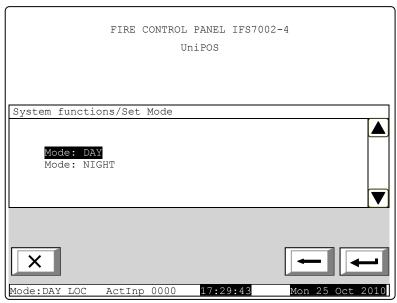
The setting of the function DAY/NIGHT must be the same for both fire control panels (Local and Rem #101). If the setting of REM #101 is NIGHT, and of the Local one - DAY, then if an event is registered for activation of manual call point from a zone in Rem #101 will make the fire control panel proceed as a whole to Fire condition phase-2.
