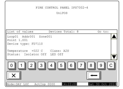
device. To edit the number press button [C], and the last entered digit is deleted.
