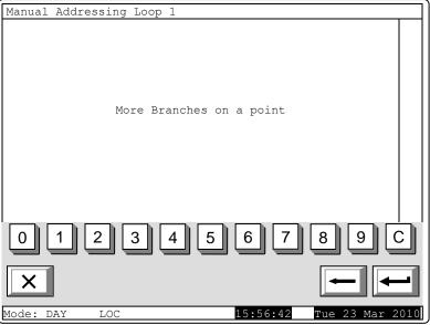
5.4. Where the provisions in sections 5.1, 5.2 and 5.3, are not met, a command for illumination of devices LEDs is sent to the uninitialized (or to one of the uninitialized) device. Depending on the result of the communication one of the following screens appears:
