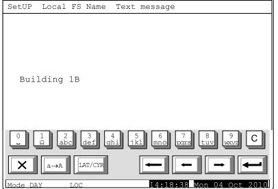
The screen displays the name of the local Control Panel Insert the name of the object (for example Building 1B).
