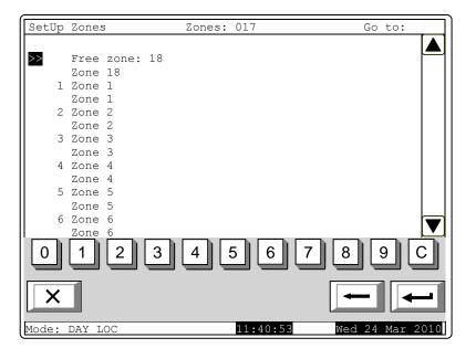
When you press a digit button the *Go to* field is activated; you can enter a random 3-digit number of a zone. To edit the number use button  $\boxed{\mathbb{C}}$  - the last inserted digit will be deleted.
