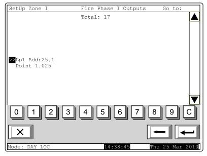
Buttons and in the right panel section are visualized if more that one free addressable output is available, and the Go to field in the heading and the digit buttons appear if free addressable outputs in more than one module are available.
