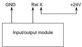
b) Diagram for connecting Input/output module to relay output
