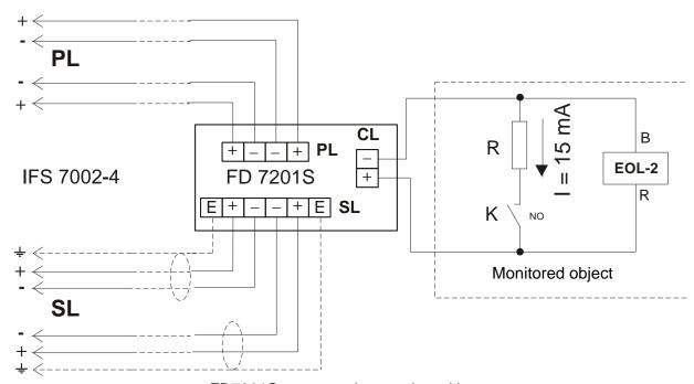
FD7201S connected to monitored input
