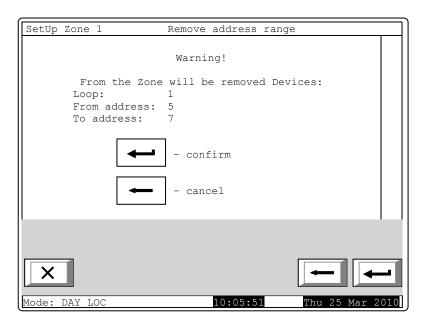
In both cases the number of the removed devices from the zone is displayed in the bottom section of the panel.
