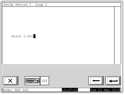
Press button to move the cursor one position to the right or to the left. Use the additional digit keypad to:
