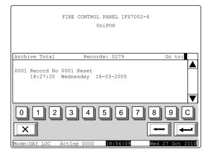
entered in the *Go to* field. To edit the number press button C, and the last entered digit is deleted.
