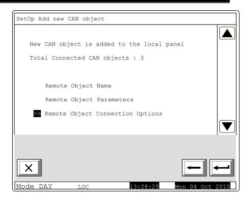
Example: To the Control Panel Building 1B, defined as a slave, are listed five connected objects with their names, CAN addresses and communication levels. Perform the setting of each CAN object separately in the menu 'Communication. Options CAN object "described below.
