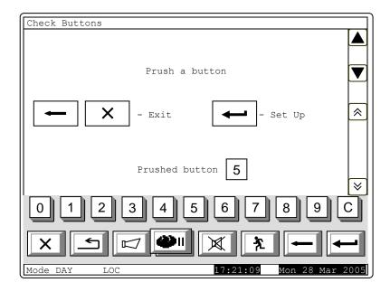
To start setting the buttons up, press button. Set up is being performed at two points on the display and is being checked at two points. Enter the function to display the first point of set up:
