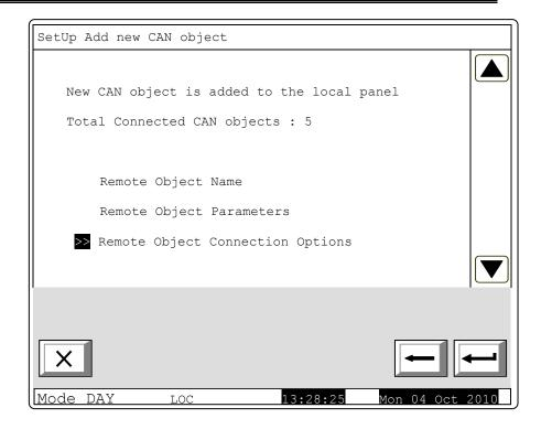
Example: To the Control Panel Administration B, defined as a master, are listed five connected objects with their names, CAN addresses and communication levels. Perform the setting of each CAN object separately in the menu "Communication. Options CAN object "described below.
