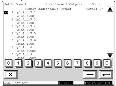
more than one output is available, and the *Go to* field in the heading and the digit buttons appear if more than 7 outputs associated to the zone are available.
