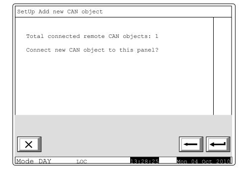
• A name of the remote object can be assigned using the menu displayed above. The name is a random one (up to 20 symbols) and is not mandatory the same name given in the local parameters of the remote object.
