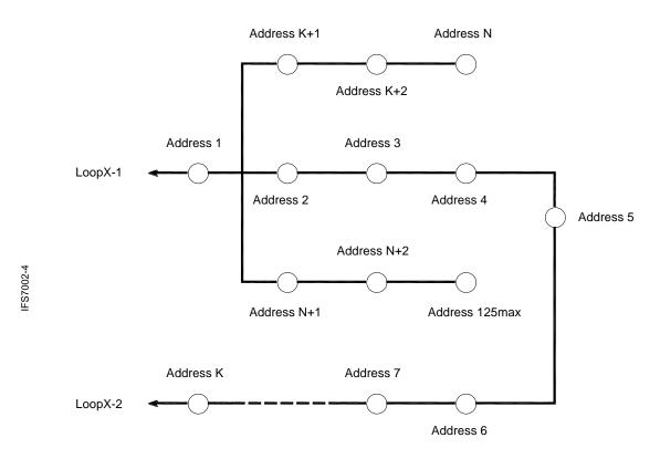
e) Improper connection of Fire alarm loop branches (two branches are connected between two addressable devices)
