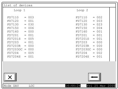
Notes: Only swithed on loops can be initialized, which are in automatic addressation mode. Where a loop is set to manual addressing mode, then the clean initialization is always unsuccessful. To make it successful, switch off the loop in manual addressing mode or to change in automatic initialization.
