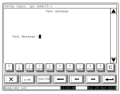
moves to the next position to the right. If you press another button during this 1 second, the cursor first moves one position to the right and then the new symbol is inserted. The maximum length of the message is 40 symbols. If you press a button after a 40-symbol message is already entered, the text will not be accepted and the symbol will not be inserted (the cursor moves one position to the right if the end of the text message is not reached yet).
