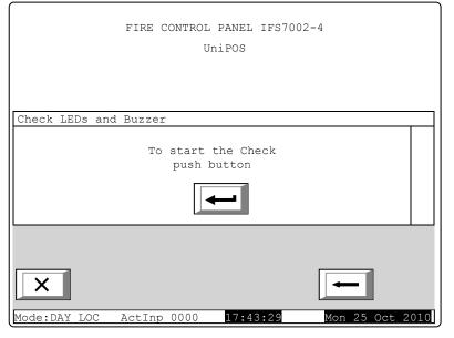
Press the button once again to discontinue the check-up operation; the LEDs and the local sounder restore their initial state.
