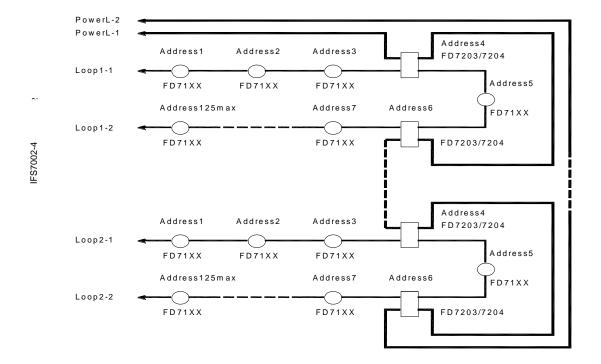
b) Configuration of Fire Alarm Loops without branches and Power Loop (recommended)
