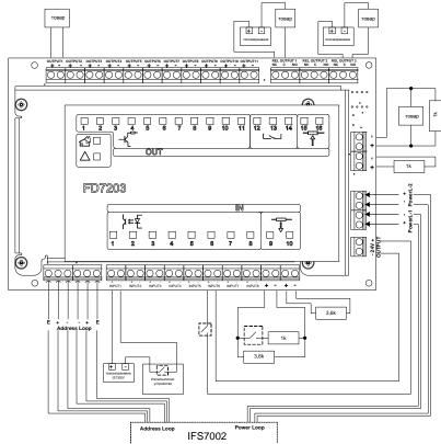
Input-output device FD7203 (10 inputs/16 outpust) Cable Connection to panel IFS7002 four signal loops
