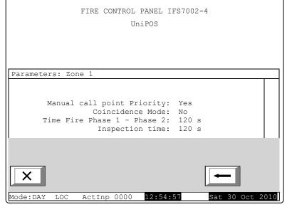
the zone will enter Fire Condition Phase 1 upon activation of at least two low priority fire detectors;
