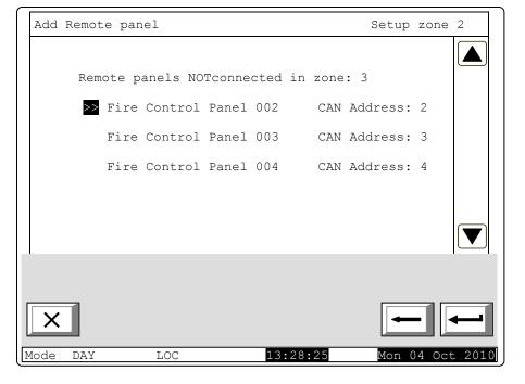
Instruction Manual Page 155 Revision 6/01.17 Of 163 Upon selecting a Control Panel (Example: Fire Control Panel 02), the number of the Remote Panels is automatically reduced.
