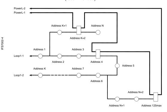
c) Configuration of Fire Alarm Loop with branches and Power Loop (Proper connection)
