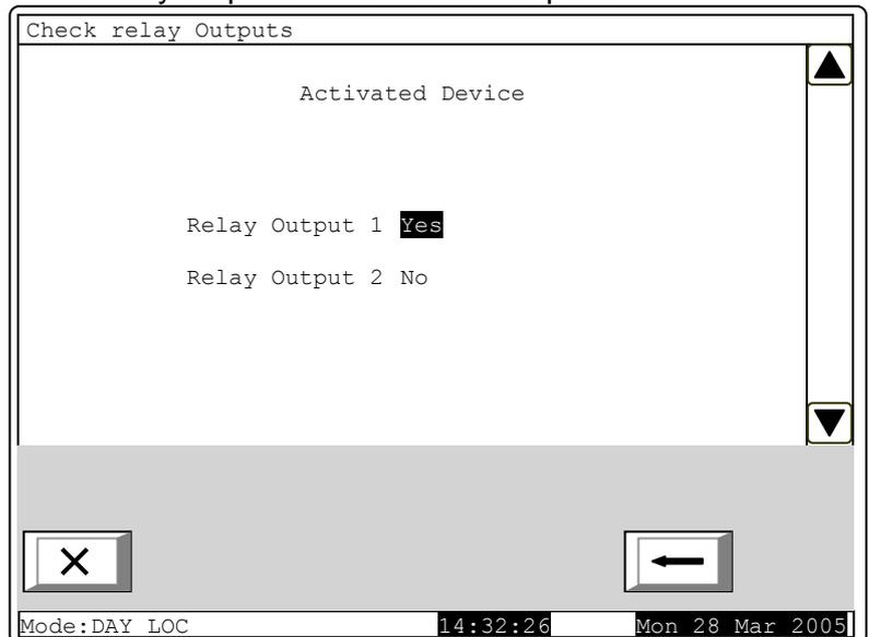
At the activated relay output appears the message *Yes* in inversive colours; at the relay output not activated yet appears the message *No*, in general colours.
