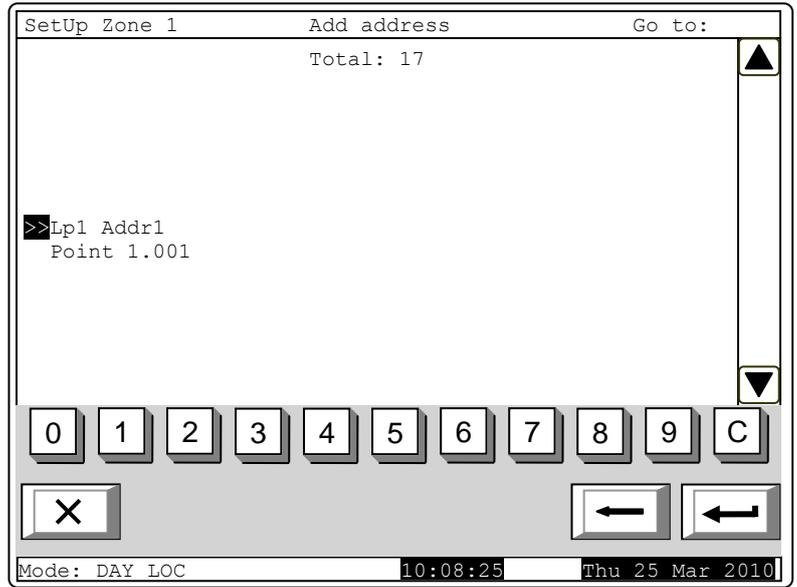
When you press a digit button, the *Go to* field is activated; you can enter a random 3-digit number for a device in the field. To edit the number push button
