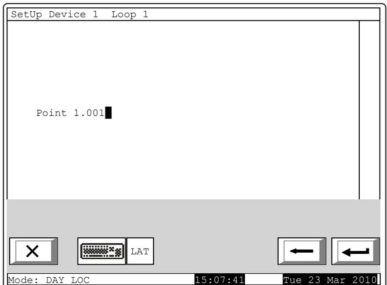
To edit the text use the buttons having symbols – when you press a button, the symbol appears over the position of the cursor, and the previous text and the cursor move one position to the right
