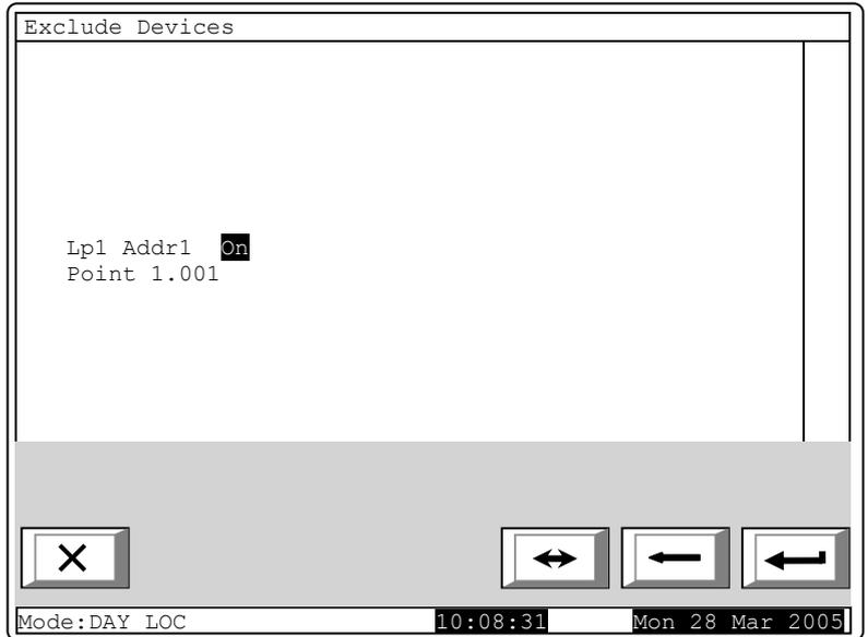
The status of the device is displayed in inversive colours. Change the status by pressing button
