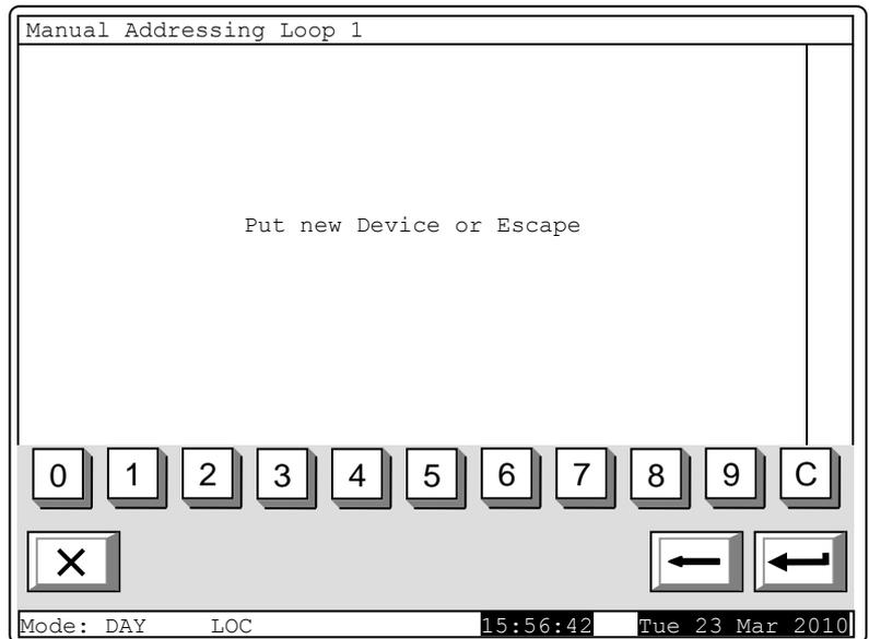
5.3. In case two or more uninitialized devices are detected in either of the loop lines, i.e. more than one branch exists at one point and devices without addressing are detected in more than two branches (in the loop and in more than one branch) the following screen appears:
