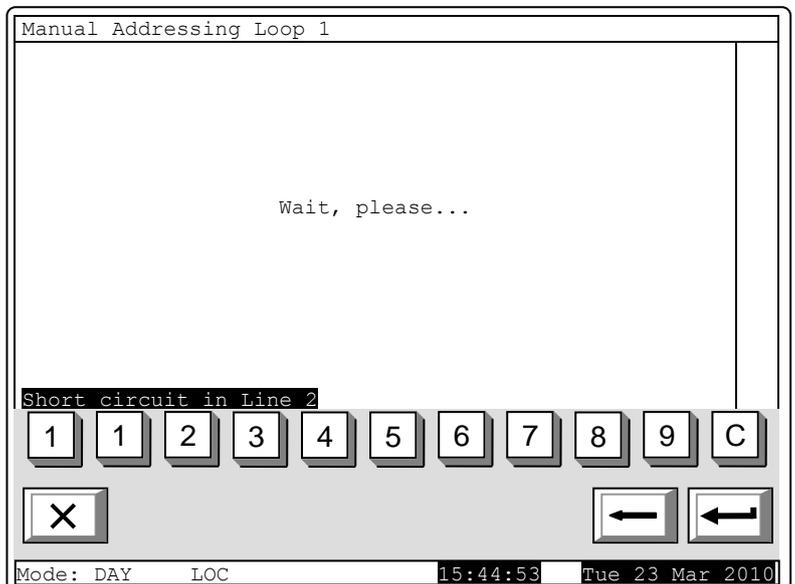
4. Check for availability of any disabled devices. During the check in the bottom right corner is displayed the counter for devices (1 to 125). Where a disabled device is detected, a command for illumination of its LEDs is sent. Depending on the result of the communication with the device, one of the following screens appears:
