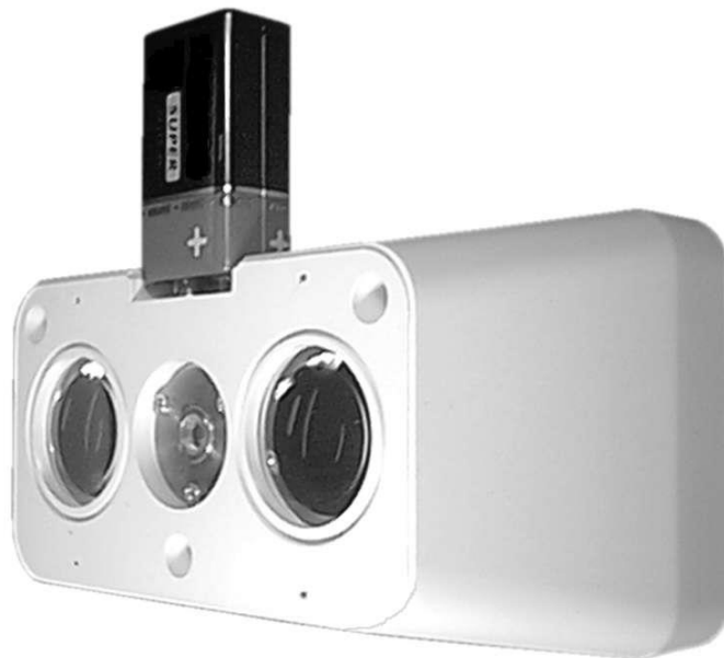
Fig. 2. DOP-6001 detector during optical path alignment
