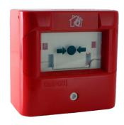
The Manual Call Point FD3050 is designed to release a signal for a fire condition to the Fire Control Panel upon manual activation by breaking the glass on the place signed with arrows. The light indication for activating the manual call point is provided by a red LED. It can be tested by a special key without operating the break glass.
