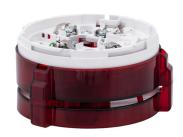
The **Sounder Base 7205** is an analog (non-addressable) fire alarm sounder and can be used together with all Unipos addressable detectors with built-in remote indication control. Sounder base 7205 is power supplied directly from addressable loop.
